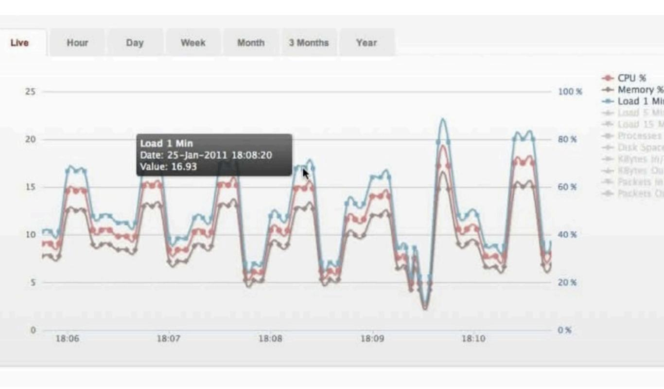
We use it for our (ve) stats feature Runs on each physical server and collects data about all running virtual servers Can send to multiple 'collector' servers that use RRD's No i/o load on any local boxes x Collect
