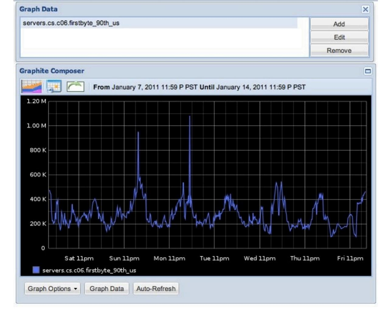
mod\_log\_firstbyte in apache is simple but useful Adds a new counter that tells you (in microseconds) how long it takes to start serving the first byte of content.
